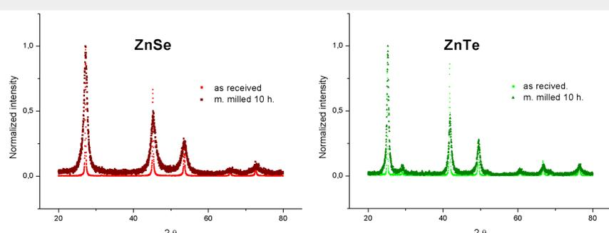
Figure: XRD patterns for ZnSe and ZnTe powders as received and after 10 hours of mechanical milling.
