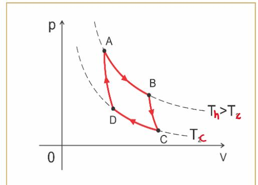
$$W_{BC} = \frac{P_B V_B^\gamma (V_C^{-(\gamma-1)} - V_B^{-(\gamma-1)})}{\gamma - 1} = (P_C V_C - P_B V_B) / \gamma - 1$$
